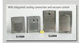
Chillvents are a simple and cheap tool to evacuate air and gases from dies. Very often they are made internally by the toolmaker.
